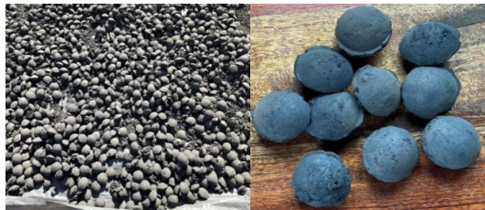
Fig. 3 Pillow-shaped briquettes produced under low-pressure briquetting technology.
